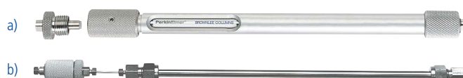
a) NewGuard cartridges directly coupled to a 220 mm MPLC cartridge (with union 07150018) b)connected externally to a 250 mm conventional column with a stand alone holder (07150001).
